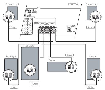
Connect each speaker using the color-coded speaker cable. Match them to the colored labels above the speaker terminals.
